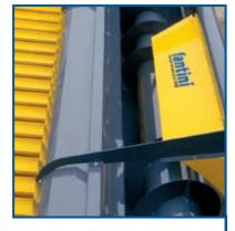
Feeding Aguer The intake Auguer perfectly guides the flower heads into the feed rake conveyor.
