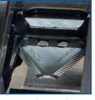
**Cutting System** The gear box and the whole cutting system are built with high quality materials and components. The divider points have been designed to ensure exceptional picking speed and to minimize product loss.
