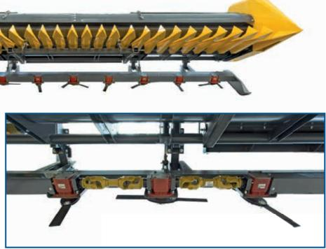
The Independent Row Unit Head can be equipped with a Stalk Chopper Kit. The cutting system is composed of blade discs with mechanical gearboxes and it covers the entire harvesting length. A cardan shaft activates the system mechanically from the right side of the transmission channel of the combine. The adjustment of the cutting height is hydraulically driven from the combine cab.
