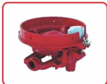
**Seed Distributor:** by disks with selected hole offering precision and efficiency.
