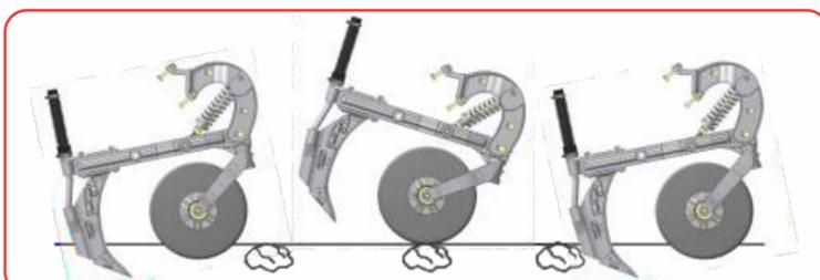
Feeling the need of several producers who cultivate rocky lands, VENCE TUDO has developed the most efficient penetration and ground attack system. Baptized and patented "stone Jumper" a simple name which exemplifies in a practical way it is essential operation to a uniform and much more efficient planting, ensuring better germination and significantly avoiding breaks and stops, common in these soil situations, reducing time and costs in the plantation process.
