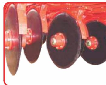
**Seed sowing:** the seed sowing system is thought two mismatched disks mounted in "V" shape with 13" and 14".
