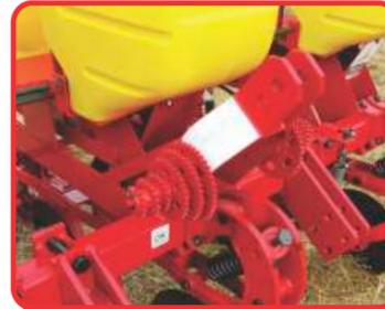
**Transmission Adjustment:** by a combination with sprockets, the sprockets are fixed in the easy place in the frame.
