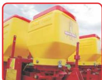
**Seed Bin:** polyethylene bucket type for thick grains, with 25 kg capacity per row.
